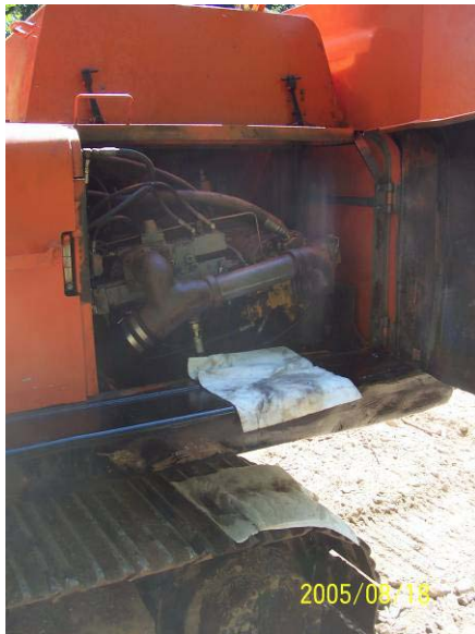
Photograph 6. A small hydraulic leak occurred when preparing the left bank haul road. All oil was contained.
