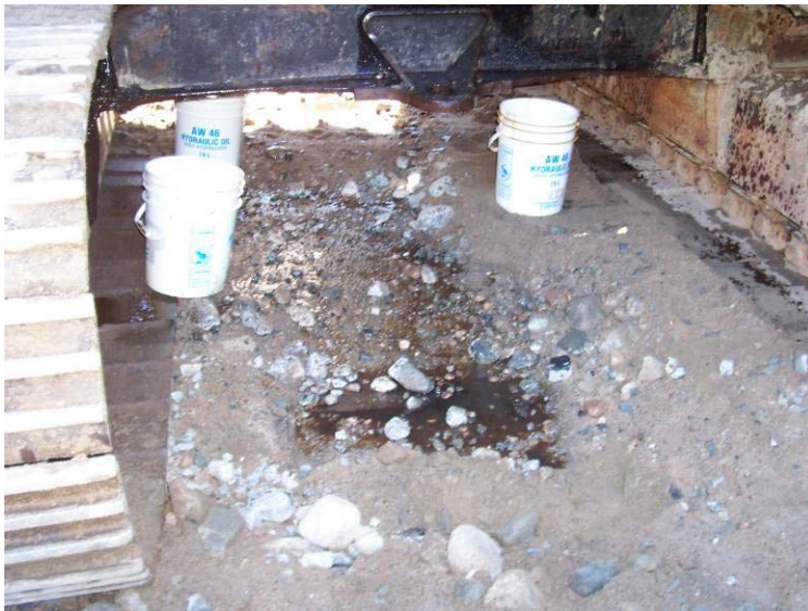
Photograph 14. Hydraulic leak on gravel bar at the Anderson site on August 25, 2005.
